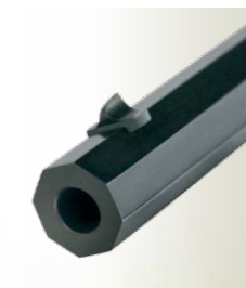
The front sight of the High-Wall Sporting model is dovetailed into the octagonal barrel and can be drifted for windage.
