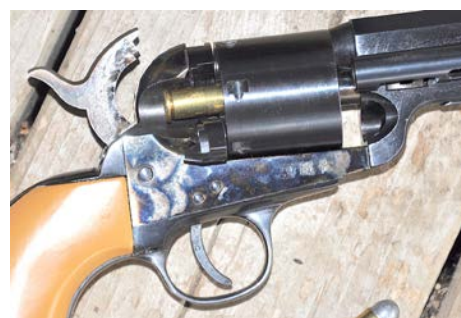
LOADING CHANNEL MILLED IN PERCUSSION REVOLVER RECOIL SHIELD TO ALLOW CARTRIDGE LOADING (AUTHOR'S COLLECTION).
