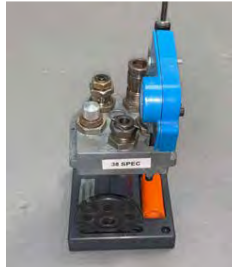
PHOTO 10 — PVC TOOL STAND FOR DILLON XL650 WITH PARTS NEEDED FOR CALIBER CONVERSION, BY KINGSNAKE.
