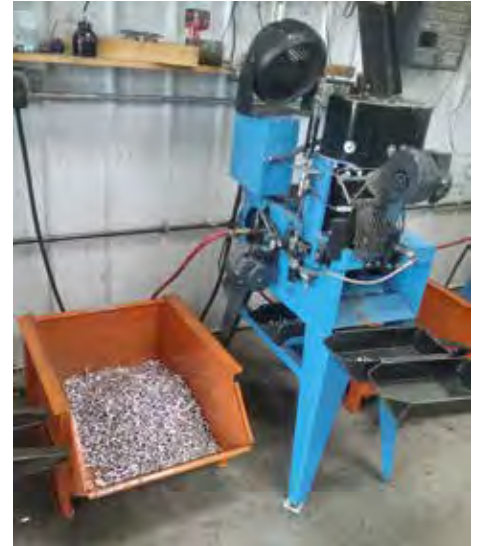
WHERE THE RUBBER MEETS THE ROAD. MOLTEN LEAD ON TOP IS SENT TO MOLDS, SETS, AND INTO THE TRAY FOR SIZING, LUBE, ETC.
