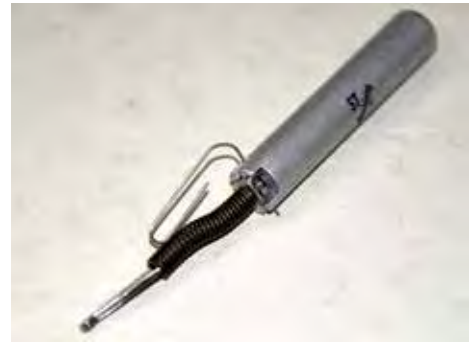
PHOTO 17 — ST MACHINING RUGER MAINSPRING COMPRESSOR WITH COMPRESSED RUGER OLD ARMY STRUT AND MAINSPRING. CUSTOM MADE CROSS-PIN NOT INCLUDED.
