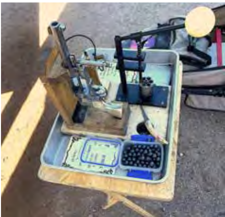
PHOTO 15 — POWDER INC. CYLINDER LOADER II WITH MATTE BLACK CERAKOTE TO PREVENT RUST AND CORROSION.
