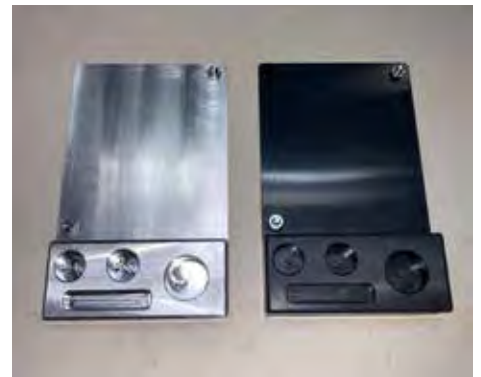
PHOTO 11 — ALUMINUM AND PVC TOOL STAND EXTENSIONS.
