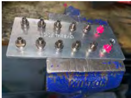
PHOTO 8 — NIPPLE CLEANING RACK WITH 12 RUGER OLD ARMY NIPPLES FOR EASY CLEANING, BY KINGSNAKE. (THE PINK ONE IS FOR THE EMPTY CHAMBER.)
