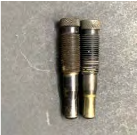
PHOTO 13 — CUSTOM EXPANDER DIE FOR RCBS COWBOY DIES. IF YOUR .38-55 BARREL NEEDS A .380 DIE, FOR EXAMPLE, RCBS DOESN'T MAKE ONE. THESE ARE CUSTOM MADE, SO OTHER DIAMETERS ARE AVAILABLE.
