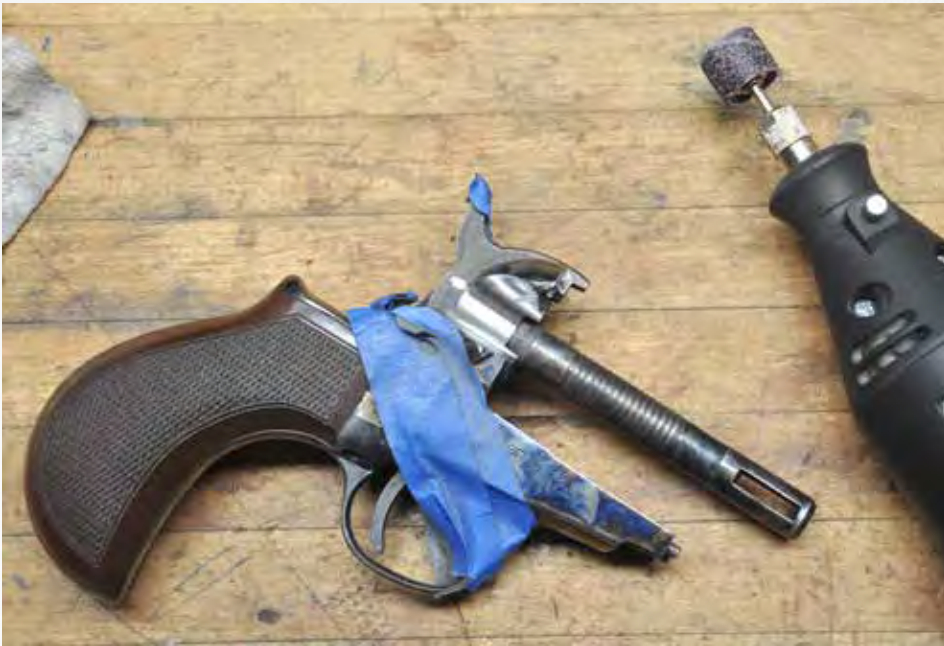
LOADING GATE CHANNEL AFTER WORK WITH THE GRINDER.
