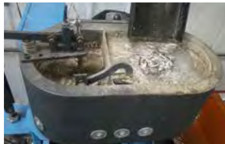
MOLTEN LEAD ON TOP OF MACHINE. LEAD IS HEATED JUST ENOUGH TO MELT, MEANING NO TOXIC LEAD VAPORS AND NO HEALTH ISSUES.
