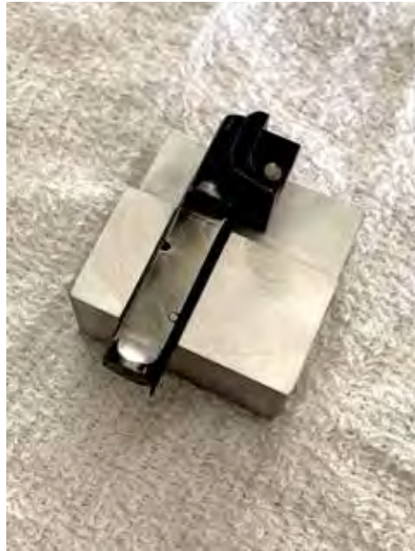
PHOTO 1 — '66/'73 BOLT BLOCK FOR REPLACING EXTRACTORS AND CARTRIDGE SUPPORT TABS, BY KING SNAKE.
