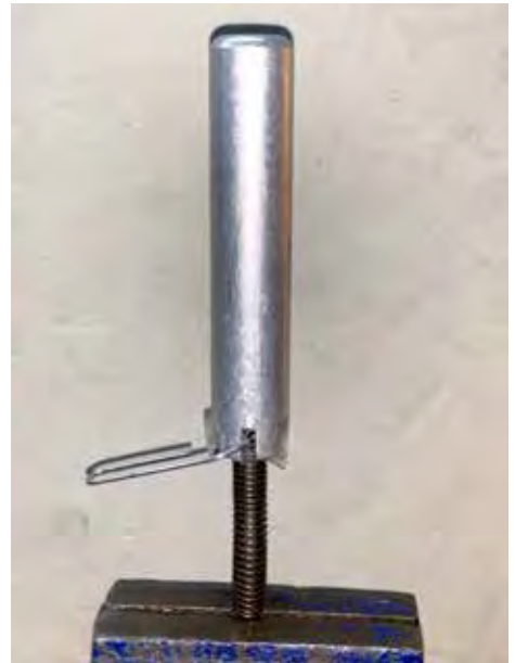
PHOTO 18 — ST MACHINING RUGER MAINSPRING COMPRESSOR MOUNTED IN A VISE FOR SPRING COMPRESSION. VISE NOT INCLUDED.
